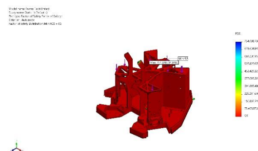
Figure 22: Vertical Load Results of analysis (FOS) of Tech United frame
