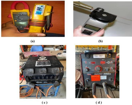
Gambar 5: (a) Multimeter fluke, (b) wire feed speed meter, (c) Loadbank, (d) Power Source
