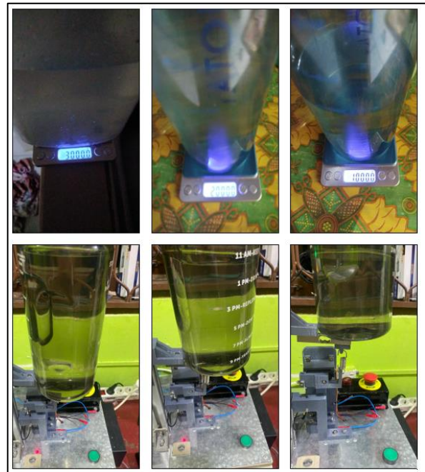
Figure 17: Load Cell Calibration Testing
