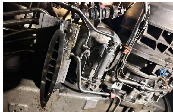
Figure 11. The Replaced Connector and the Fuel Tank Ejector After Reinstallation
