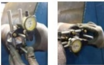
Gambar 12: Pengukuran Pitch Diameter
