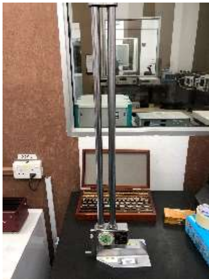
Gambar 4: Dial Height Gauge
