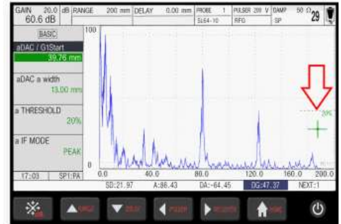
Gambar 5: Tampilan peak hasil kalibrasi
