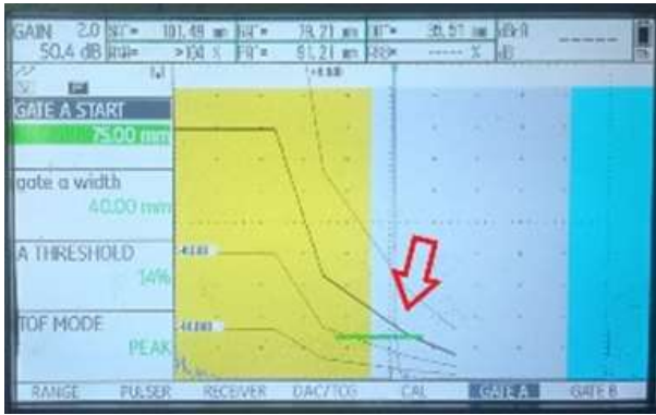
Gambar 3: Tampilan Peak Dua Back Wall Echo (BWE)
