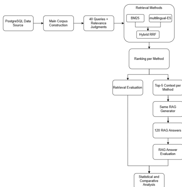
Figure 1. Main experimental workflow for comparing retrieval methods under the Top-5 RAG configuration
