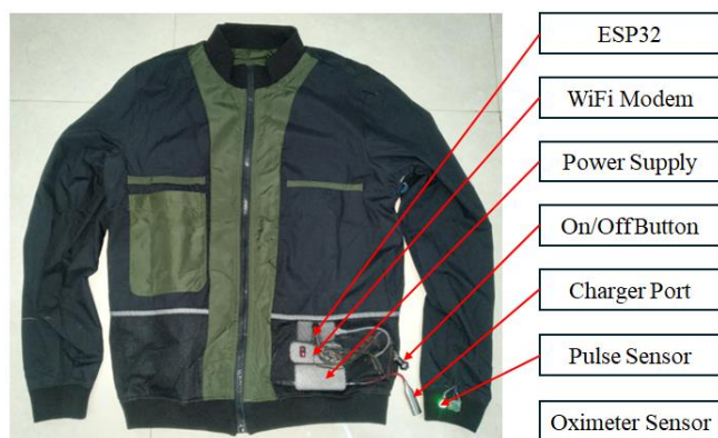
Figure 4. Interior of the jacket, front view
