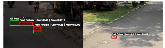
Figure 10. Representative False-Positive Cases in Pothole Detection
