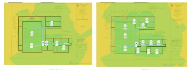
Figure 3. Third floor coverage comparison: efficient design with 6 APs (left) and ideal design with 12 APs (right)
