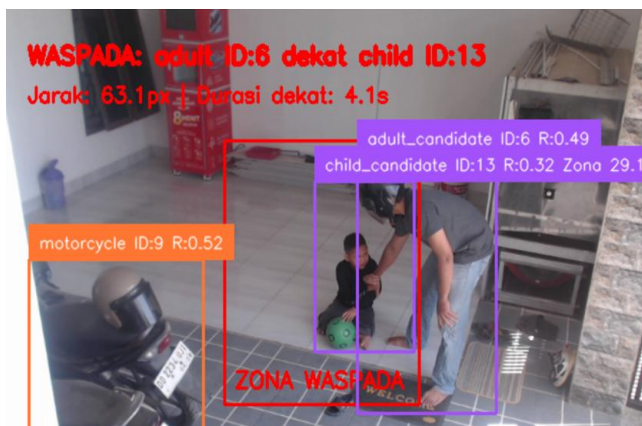
Figure 2. YOLOv8 bounding box object detection system
