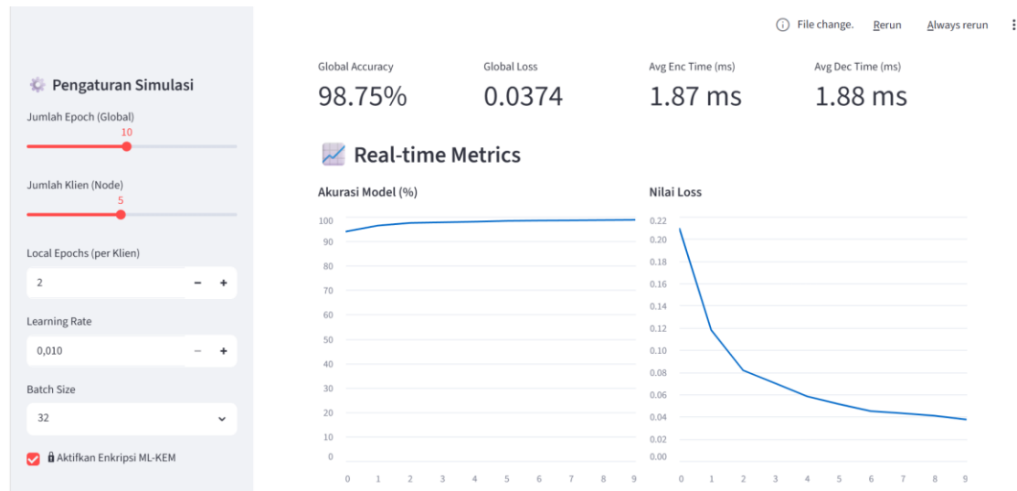
Figure 2. Global Model Convergence Curve Over 10 Rounds with the ML-KEM Protocol
