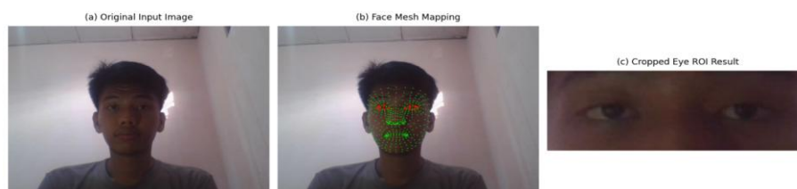
Figure 2. Visualization stages of input image processing: (a) original input image from the webcam, (b) mapping of the facial landmark coordinate mesh matrix via MediaPipe Face Mesh, and (c) the resulting isolated ROI eye-area cropping segmentation with padding space expansion
