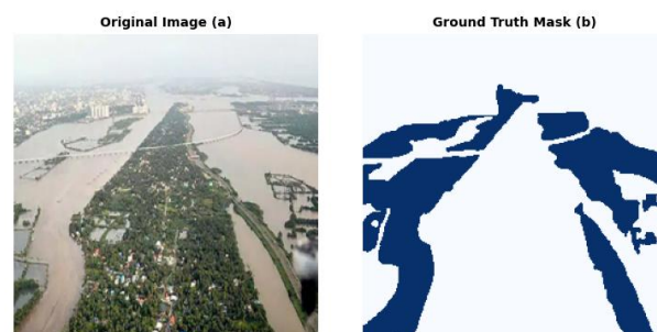
Figure 1. Example of UAV aerial imagery and its corresponding ground truth mask: (a) UAV image, (b) binary flood mask
