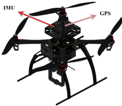
Figure 2. GPS Sensors and IMU Placement
