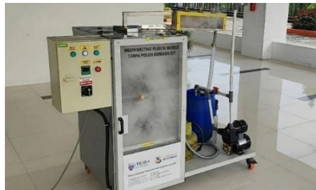
Figure 4. Realized prototype of the Mobile Plastic Melting Unit in operation (demonstrating emission mitigation).
