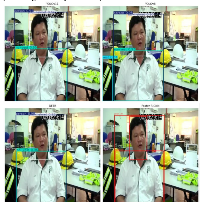
Figure 7. Detection results comparison on an indoor test image depicting an individual without required PPE (no-helmet, no-vest), with PPE items present in the background.
