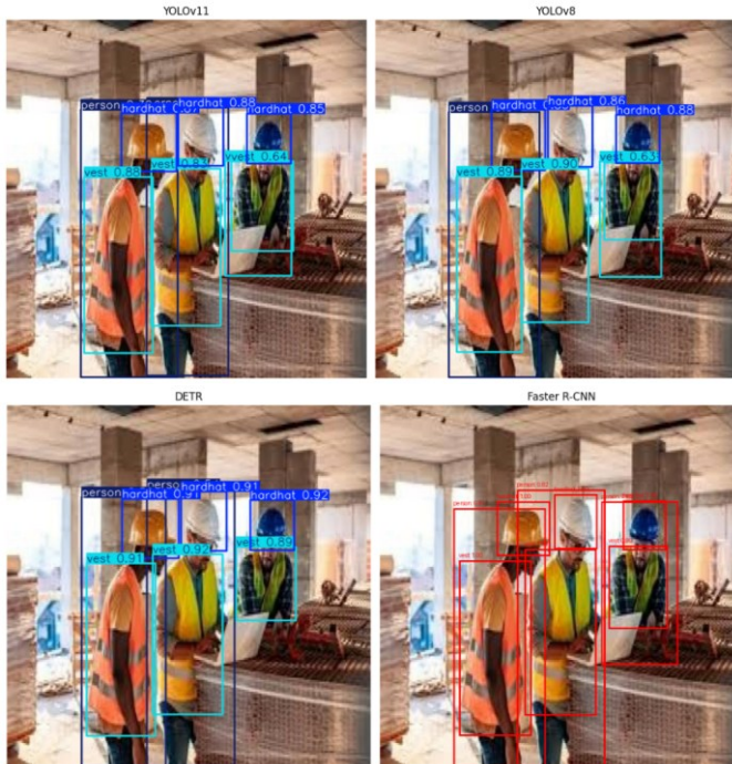
Figure 5. Visual comparison of detection results on a test image featuring workers in close proximity with partial occlusion.
