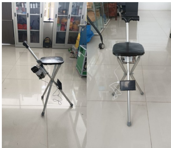
Figure 15. Final design of the smart cane prototype showing the ergonomic handle, foldable seat, and embedded electronic components
