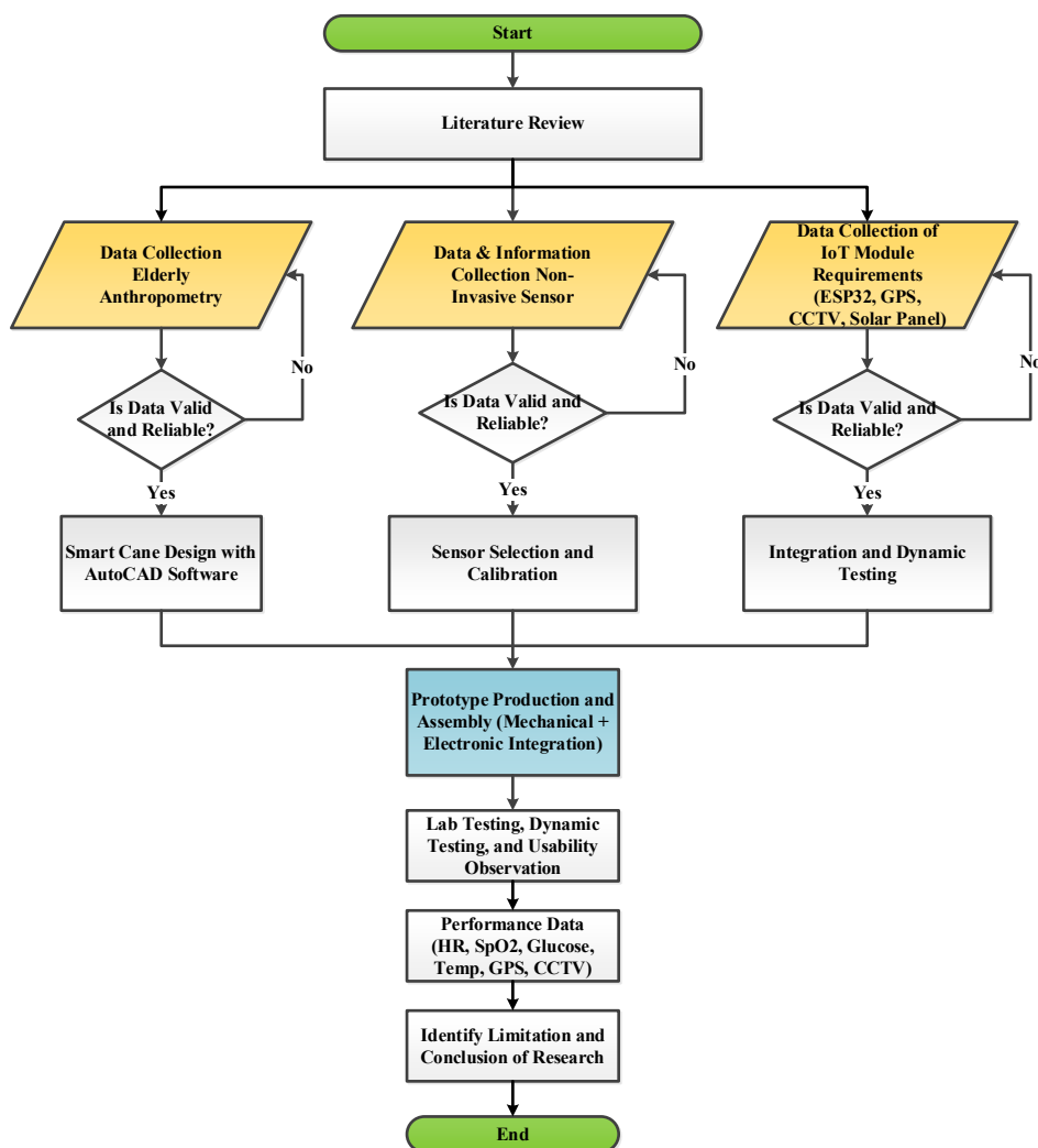
Figure 1. Research flowchart of IoT-based smart walking cane development.
