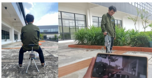
Figure 16. Field testing of the smart cane outdoors with live data monitoring and CCTV streaming connected to the Blynk platform
