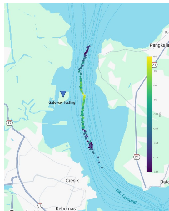
Figure 3. Initial Signal Characterization Based on RSSI Values in the Madura Strait Testbed
