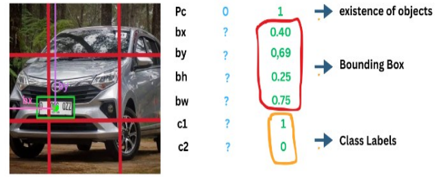
Figure 3. How YOLO works [17]
