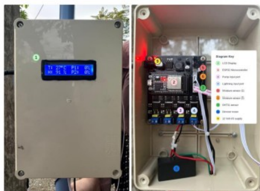
Figure 1. Detailed IoT Monitoring System [9]
