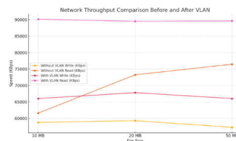
Figure 9. Network Throughput Comparison Before and After VLAN
