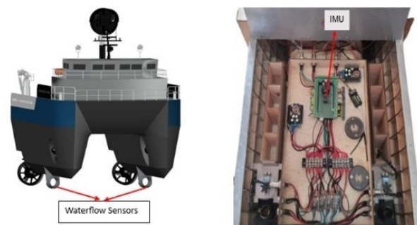
Figure 2. Waterflow Sensors and IMU Placement
