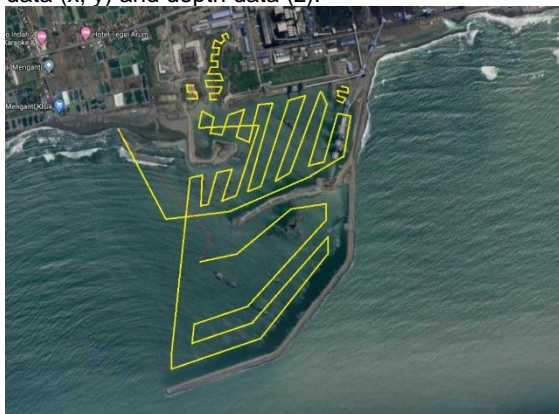
Fig 4. Bathymetry survey trackline
