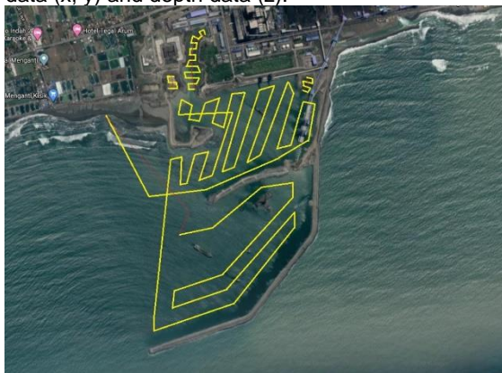
Fig 4. Bathymetry survey trackline
