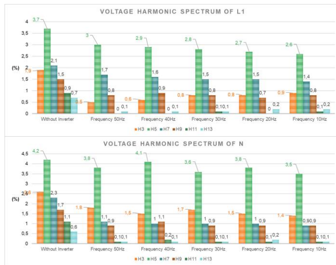
Figure 6. Spectrum Harmonic Voltage L1 &amp; N
