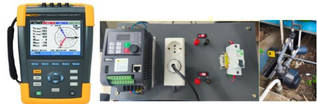
Figure 1. Fluke Power Quality 434, VFD 1 Phase & Motor
