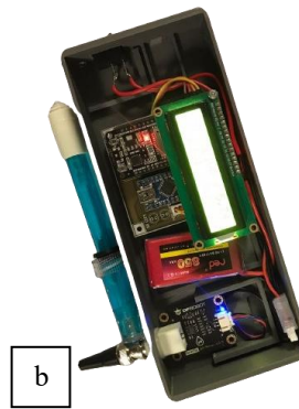
Figure 2. (a) Mechanical design of the portable GERD diagnostic device with ergonomic features for user comfort; (b) Detailed mechanical system incorporating a beaker glass for saliva samples and sensor insertion for pH measurement (units in cm)
